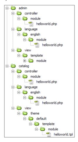
So now you know the basic directory structure of OpenCart module. The file structure is divided into two sections **admin** and **catalog**. The admin folders and files deal with the setting of the modules and data handling, while the catalog folders and files handle the frontend.
